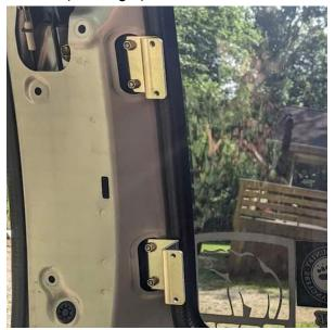
Step 5 -On the latch side, take the "F" mounting bracket and install the "A" bolt through the lower hole, and place the 2x "B" washers on the backside of the bracket; the window latch assembly has a curve to it, and these act as spacers to tighten the mountain bracket evenly.
