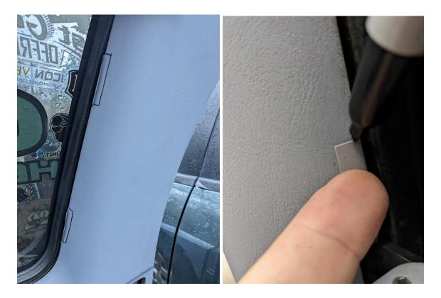
Step 4 - Using the "C" spacers, install 1 thick spacer on the bottom, and one thin spacer on top of that to each pair of studs on the hinge side of the window. Install "E" brackets on top of that, and either reuse factory flange nuts or use the provided "D" Nylock Flange Nuts. Tighten to 6-7ft lbs (hand tight).
