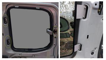
Step 3 - Remount your interior door panel, and mark the edges of the paper templates on the door frames. Do not cut them at this time. Once door panels are marked, remove paper templates / associated hardware.
