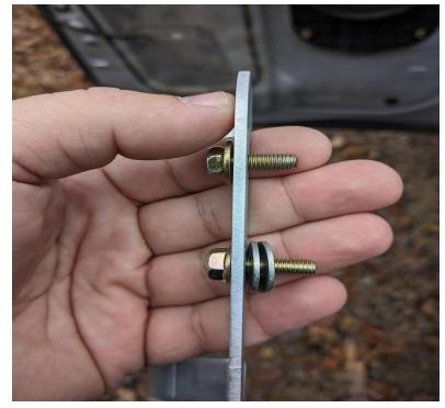
Step 6 - With the brackets now in place, test fit your door panel, and begin trimming the interior of the door panel, and the notches, to fit over the new brackets and hardware. Pics attached as an example. After each trim, continue to reinstall the door panel until you have a satisfactory fit.
