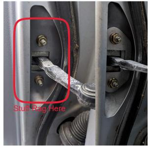
3: Slide plate over the bolts, and reattach nuts over the top. Snug tight by hand, but do not apply excessive force (or God forbid, use an impact wrench). All finished!
