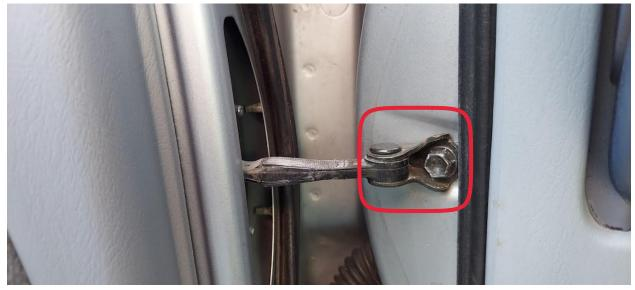
2: Open the door fully (and keep it there), and remove the 2 nuts; make sure not to drop them inside the door. They are recoverable, but you have to remove your door panels/trim to access where they fall down to. A small rag stuffed in the bottom of the opening should catch anything that falls.
