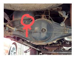
Install the new breather assembly. Snug down with a 14mm wrench.
