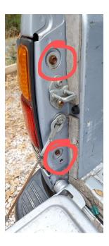
Behind the tail light, you'll see a threaded hole. Using the 4mm Allen Wrench (or T25) snug the zip tie holder into place. Thread a zip tie through, and zip the breather into position.
